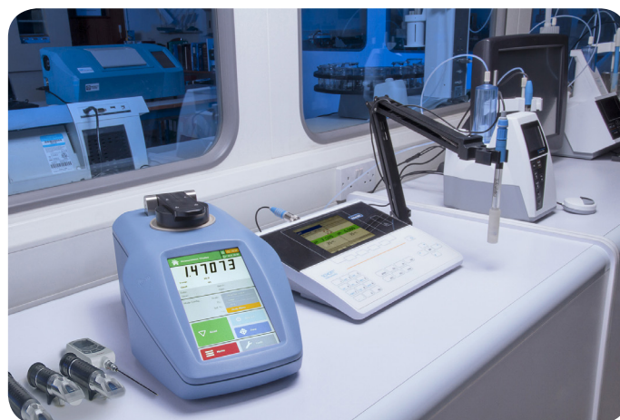
Fig. 1: RFM900-T Series Peltier temperature controlled refractometer in the laboratory with associated instrumentation available from Xylem
